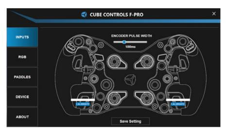
The process is simple: when connecting the F-PRO for the first time, the clutches could be not recognized by the program and pressing them would not make a difference.
