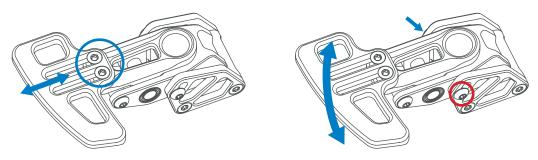
Caution: do not use a tightening torque higher than 5 Nm.
