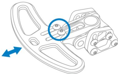
Reach can be adjusted by slightly loosening the two screws highlighted as the right picture and the two on the opposite side of the shifter as pointed by the small arrows, then rotating the lever body upwards/downwards. You may need to apply a bit of force.
