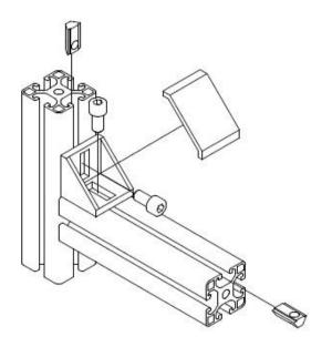
In some cases you will have to break off the guiding feet of the brackets. That can be easily done by prying them with a screwdriver.
